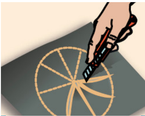
Figure 1 - First piece of Mapethene LT to be cut to suit the diameter of the member passing through the surface
